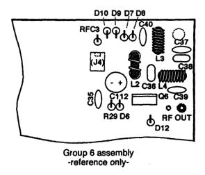
Q6 (2SC2078 or equivalent) is installed with the metal tab to the rear (or 'top' when viewed from directly overhead). When viewing the board from the front edge (U1, U3, and U4 nearest you), Q6's labeling must be viewable.
