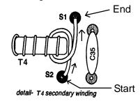
5) Install this lead-end in S1 and solder.
