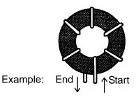
This toroid is wound with 6 turns of #26 gauge enameled magnet wire.
